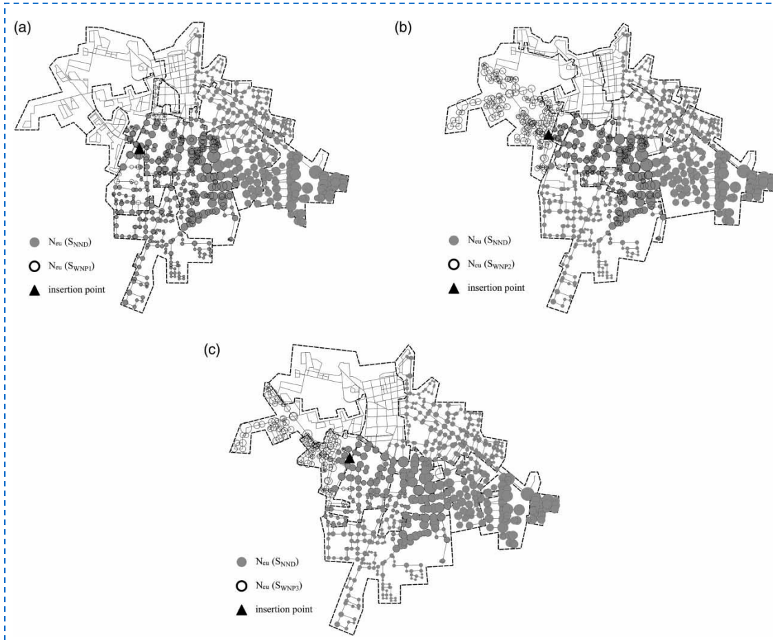
Comparison of exposed users (Neu) between original network and three partitioning layout with different weights.
